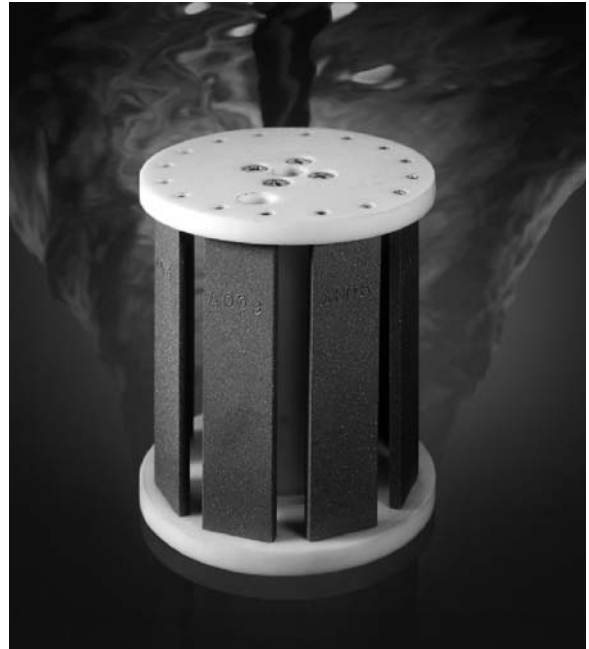
NOTE 1—Gaps (typically 0.85 cm ± 0.01 cm) between the coupons introduce localized turbulence.
